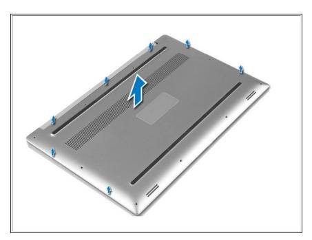
• Pry the edges base cover and lift it to remove it from computer.
