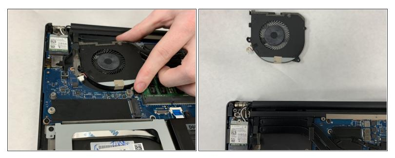
• Carefully extract the fan from its housing bed. It should remove easily if all parts have been disconnected.
