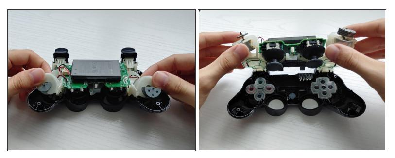
Lift off the plastic housing holding the motherboard, battery, and vibrating motors.
