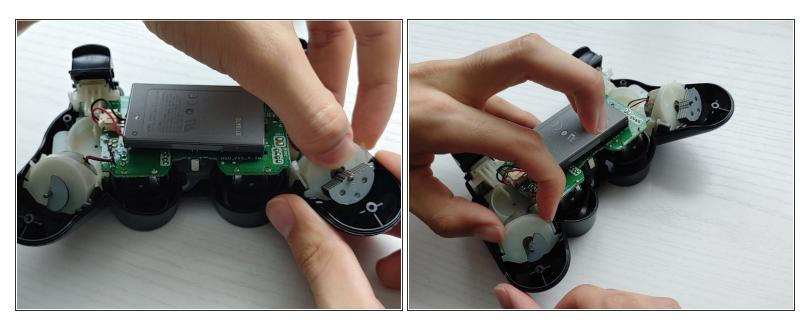
• Unclip the vibrating motors.
