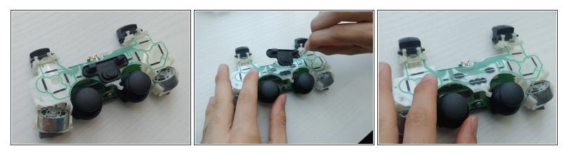
• Remove the rubber buttons with a pair of tweezers.
