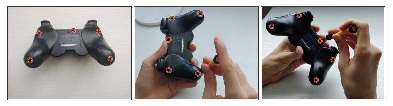
• Use a Phillips #1 screwdriver to remove the five 7.2 mm screws securing the rear cover.
