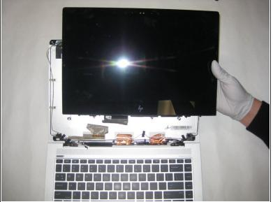
Lift the display up and out of its housing.
