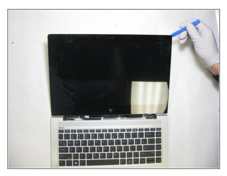
Wedge an opening tool between the display and the chassis, gently prying around the perimeter until the display completely releases.
