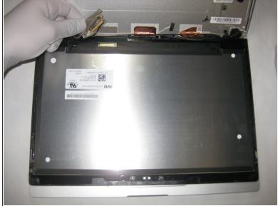
Lift the metal arm, then pull the display ribbon cable directly out of its port.
