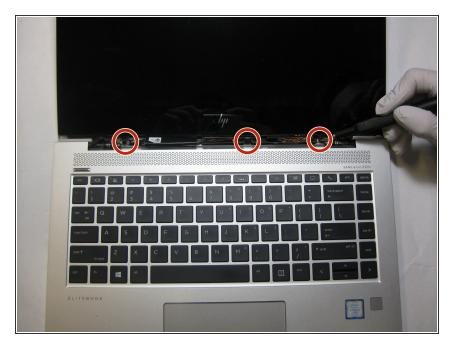
Use a Phillips #00 screwdriver to remove the three 5 mm black screws that securing the dispaly.
