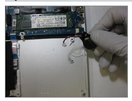
• Remove the coin cell battery.
