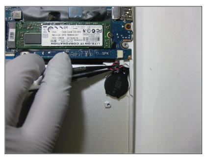
• Carefully disconnect the coin cell battery cable located under the motherboard.
