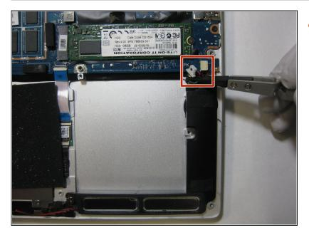
Carefully disconnect the pin connector from the right side of the speaker assembly.
