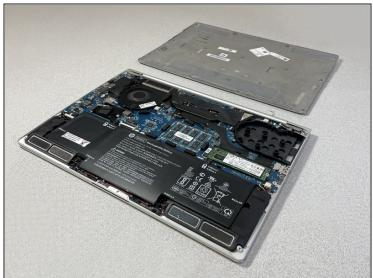
• Lift the back cover up and off the device.
