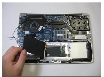
Peel back the foam cover to reveal the underside of the trackpad.
