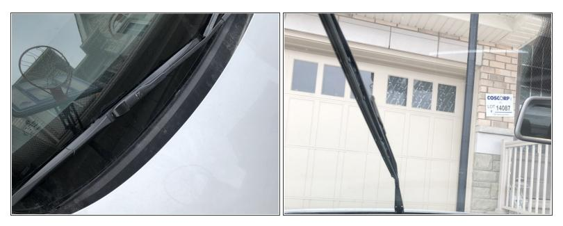
• Lay the wiper arms back down onto the windshield, start the car and test the windshield wipers to make sure they've been replaced successfully.
