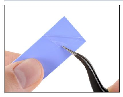
Use a pair of tweezers to peel one side of protective film away from the remaining thermal pad.
