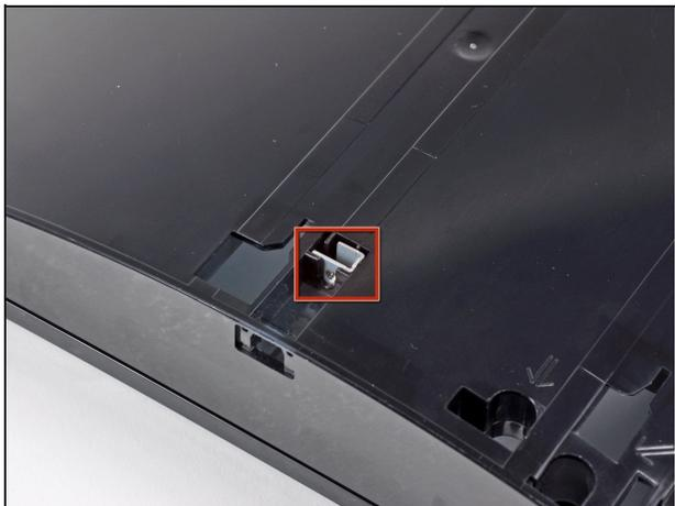
⚠ Be sure to keep track of the small metal bracket loosely held in the top cover, if equipped.
