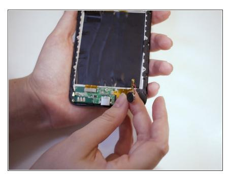
Carefully lift up the vibrator, connected to the board by two wires.
