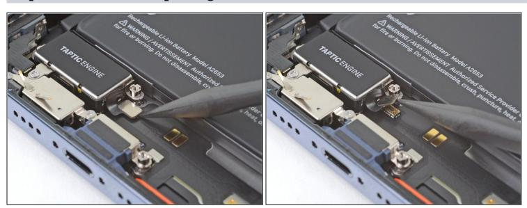
• Pry up with the pointed end of a spudger to disconnect the Taptic Engine cable.
