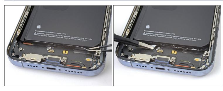
• Use a pair of blunt-nosed tweezers to peel down the two battery adhesive pull-tabs along the bottom edge of the battery.
