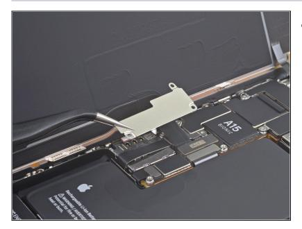
• Remove the battery connector cover.
