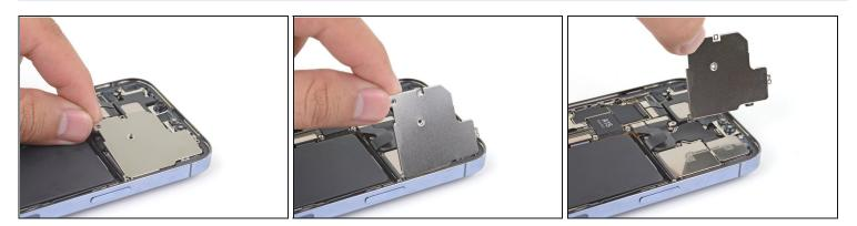
• Lift the camera cover from the edge closest to the logic board, and remove it.
