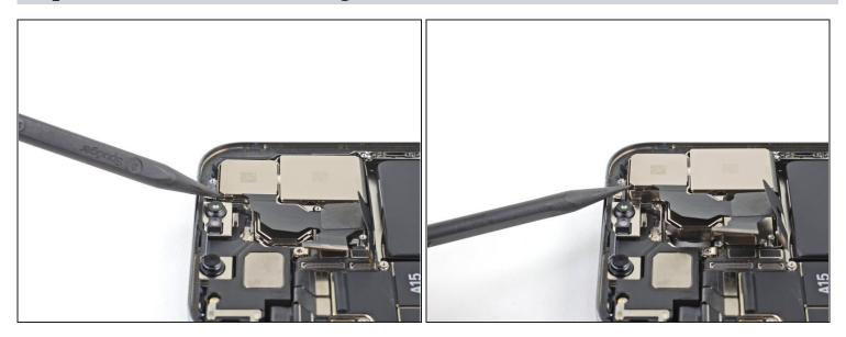
• Use the tip of a spudger to lift the camera assembly out of the iPhone.
