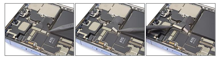
• Pry up with the pointed end of a spudger to disconnect the two camera cables from the logic board.
