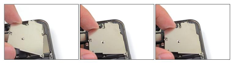
When reinstalling the camera module cover, ensure the lip along the right edge slides underneath the phone's chassis.
