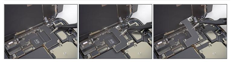
• Remove the front sensor connector cover.
