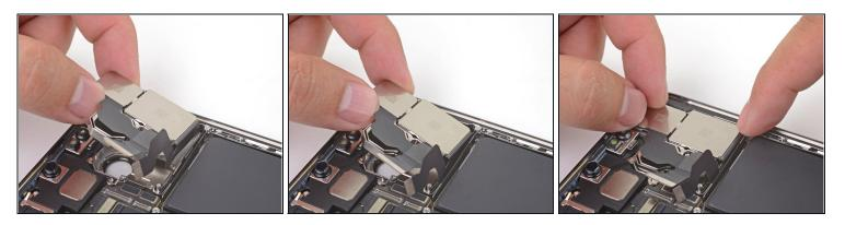
During reassembly, you'll need to insert the two camera assembly cables into the gap between the upper battery wall and lower camera wall.
