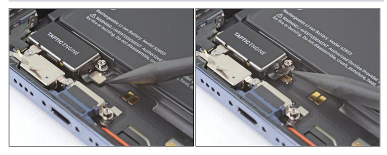
• Pry up with the pointed end of a spudger to disconnect the Taptic Engine cable.
