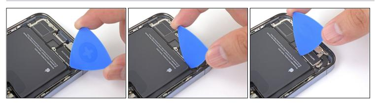
Slide an opening pick between the top edge of the taptic engine and the adhesivebacked strip.
