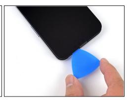
• Slide the opening pick around the top right corner of the iPhone to separate the top adhesive.
