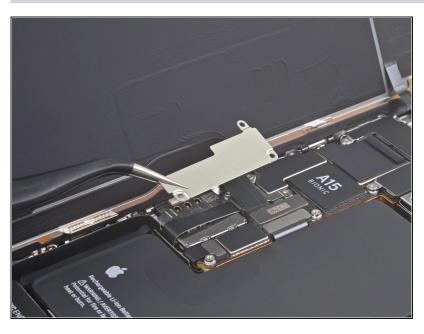
Remove the battery connector cover.
