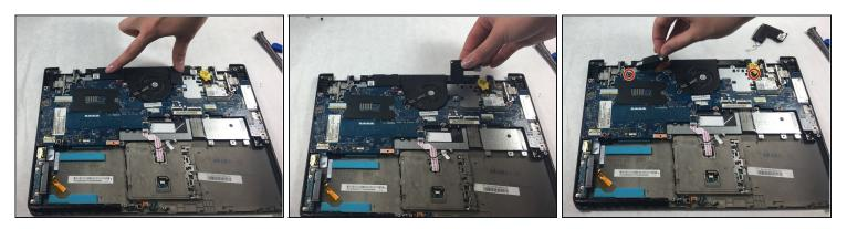
• Disconnect connectors. Use fingers to pinch and pull the connector out.
