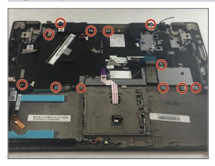
Remove twelve screws from the midframe using a Phillips #1 screwdriver.
