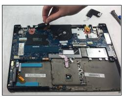
Disconnect connectors. Use fingers to pinch and pull the connector out.
