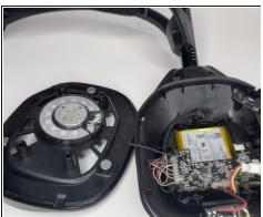
• Remove all four 1.5 mm screws using the Phillips #00 screwdriver.
