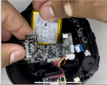
• Remove the old battery with a plastic opening tool.
