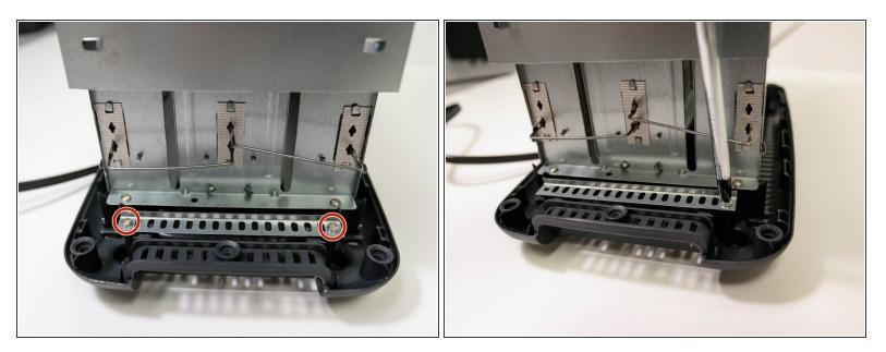
Use a Phillips 2 x 4in. screwdriver to remove the two 0.25 in. Phillips head screws. This will allow you to remove the metal bracket.
