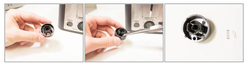
• Use a pair of mini long-nose pliers to remove the spring components from the timer knob.
