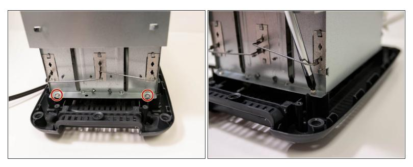
Use a Phillips 2 x 4in. screwdriver to remove the two 0.25 in. Phillips head screws. These screws secure the back of the internal housing of the toaster.
