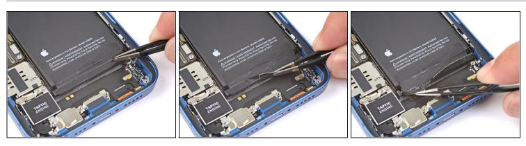
Peel up the two remaining battery adhesive pull-tabs to un-stick them from the bottom edge of the battery.
