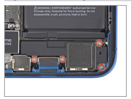
Use a Phillips driver to remove the four 1.7 mm screws securing the loudspeaker.
