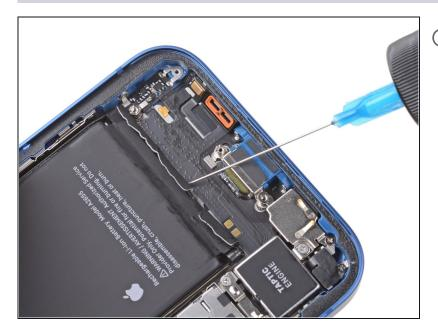
(i) Optionally, tilt the bottom of the phone up and apply a few drops of high-concentration (90% or higher) isopropyl alcohol to the bottom edge of the battery, and wait a minute. It'll help soften the adhesives, especially if the phone is old.
