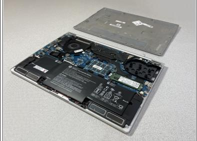
Lift the back cover up and off the device.
