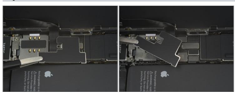
Use a pair of tweezers to remove the battery and display connector cover.
