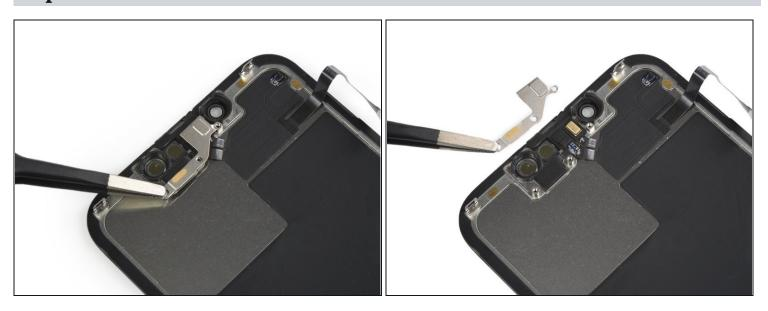
• Use a pair of blunt nose tweezers to remove the metal cover.
