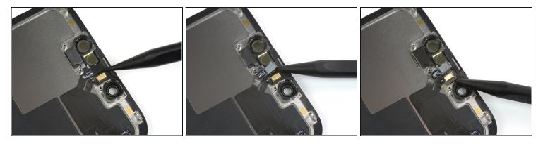
Use the pointed end of a spudger to pry the proximity sensor and the microphone out of their recesses.
