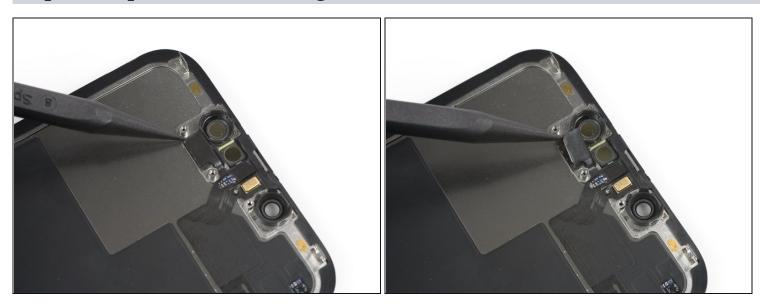
Use the pointed end of a spudger to pry the ambient light sensor out of its recess.
