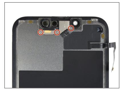
Remove the three 1.4 mm-long tri-point Y000 screws securing the sensor assembly cover.
