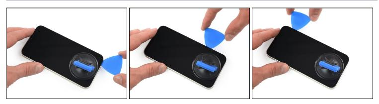
• Slide the opening pick around the bottom right corner and along the right edge of the iPhone, slicing through the adhesive holding the display in place.
