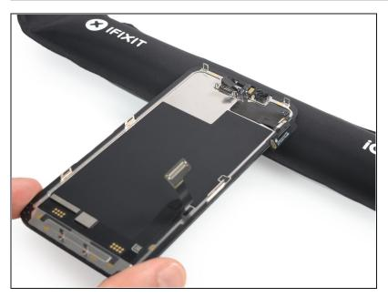
Use a hairdryer or heat gun or prepare an iOpener and apply it again to the top front of the display for 1-2 minutes, in order to soften the adhesive securing the sensors.
