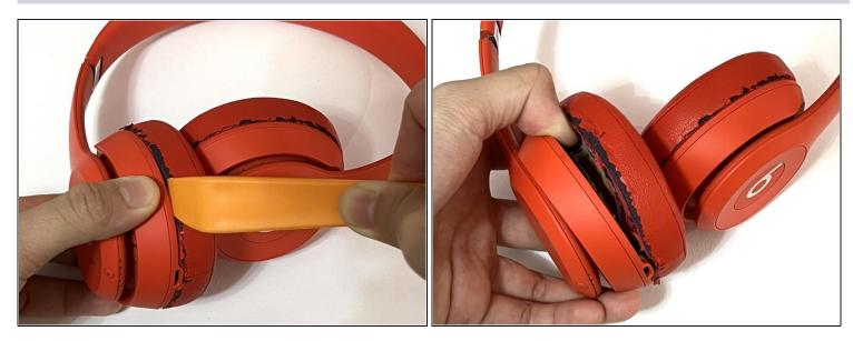
Use a halberd spudger to create a gap between the earpads and the main body.
