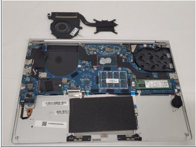
• Lift and remove the fan and heatsink assembly from the device.
