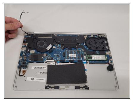
Carefully remove the wires from the clip to the left of the fan.
