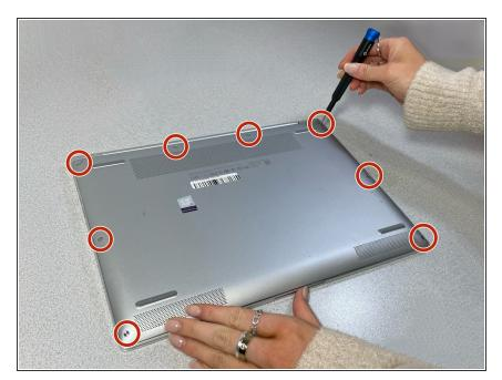
Use a T5 Torx screwdriver to remove the eight 5 mm screws securing the back cover to the chassis.
