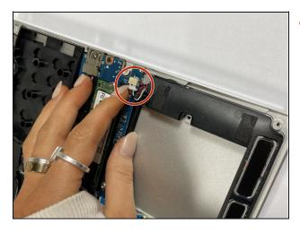
Disconnect the pin connector from the right side of the speaker assembly.
