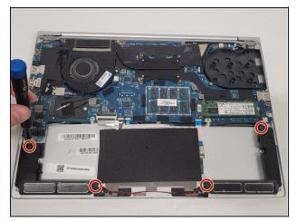
Using the Phillips #1 screwdriver, remove the four black 6 mm screws securing the speakers to the device.
