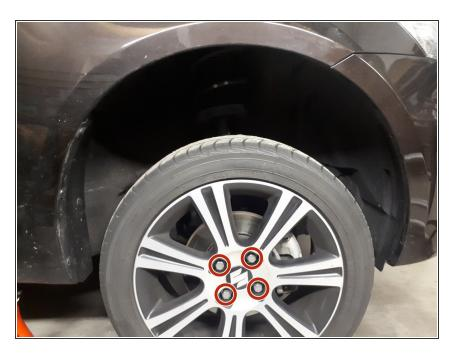
Using the 17mm socket, unbolt the wheel nuts and remove the tire from the hub.
