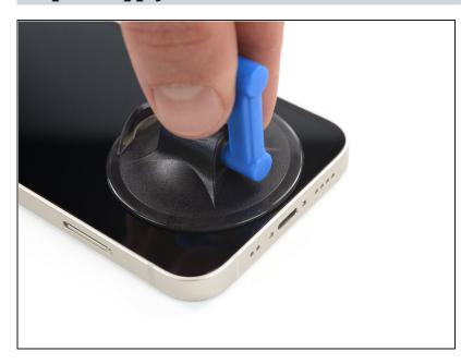
• If you're using a single suction handle, apply it to the bottom edge of the phone, as close to the edge as possible.
