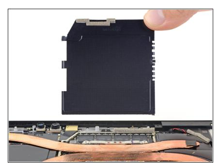
• Remove the heat sink shield.
