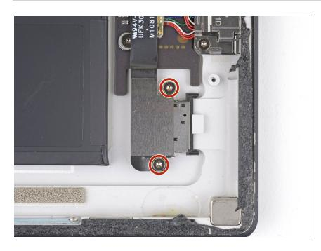
Use a T5 Torx driver to remove the two 3.1 mm screws securing the microSD card reader.
