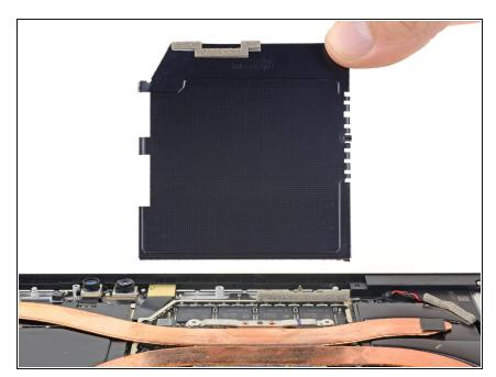
• Remove the heat sink shield.
