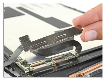
• Lift the EMI shield away from the display board and remove it.
