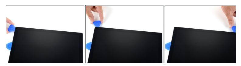
Insert a new opening pick into the bottom right corner and slide it around the corner toward the bottom edge.
