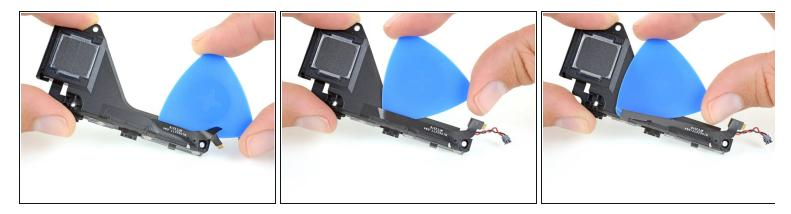
• Slide an opening pick under the volume and power button cable to separate the adhesive securing the cable to the speaker.
