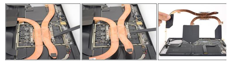
Use a spudger to gently pry the heat sink straight up and off of the CPU.
