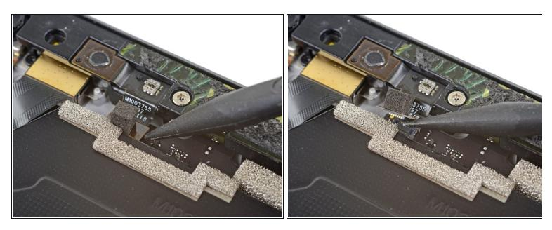
Use the point of a spudger to pry the microphone connector straight up and out of its socket on the motherboard.
