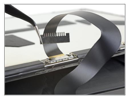
• Pull the rest of the shield off of the digitizer connector and remove it.
