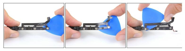
• Slide an opening pick under the volume and power buttons to separate the adhesive securing the buttons to the speaker.
