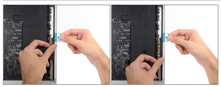
• Use your finger to smooth out the strip. Make sure it is neatly aligned with the right side of the frame and that it sits flat.
