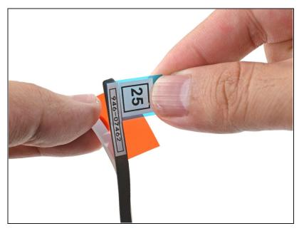
Grasp the red pull tab on strip 25 and pull to separate about 2 inches (5 cm) of white backing from the strip.
