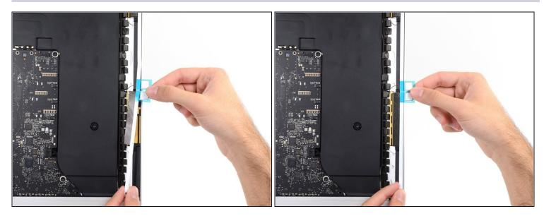
• Align the lower portion of the strip with the right edge of the frame, and stick it down.
