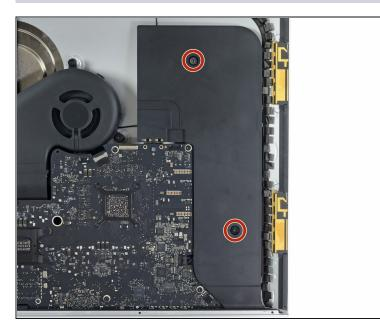
• Use a T10 Torx screwdriver to remove the two 10 mm screws securing the right speaker.
