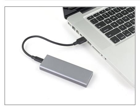
The drive is now ready to be connected to your computer with either of the included USB cables.
