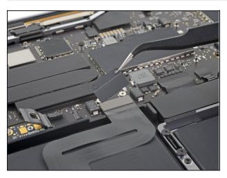
Remove the trackpad cable connector bracket.
