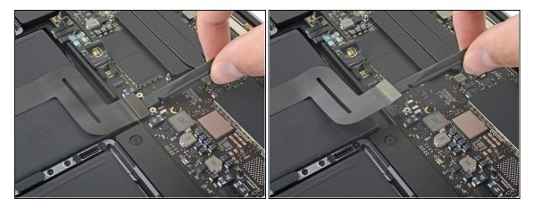
• Use a spudger to disconnect the trackpad ribbon cable by gently prying its connector straight up from the logic board.
