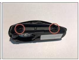
Release the four clips that have been revealed on the sides
