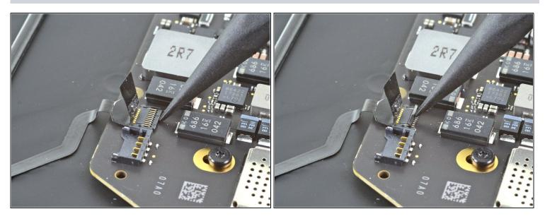
Use the pointed end of a spudger to lift up the small locking flap on the microphone cable's <u>ZIF</u> connector.
