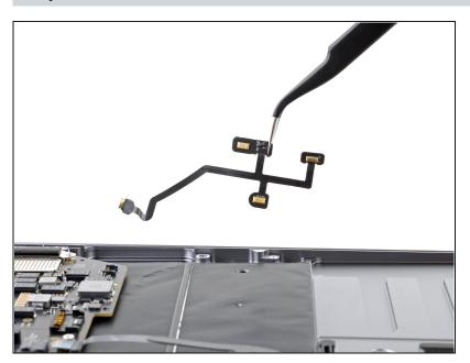
• Remove the microphone array.
