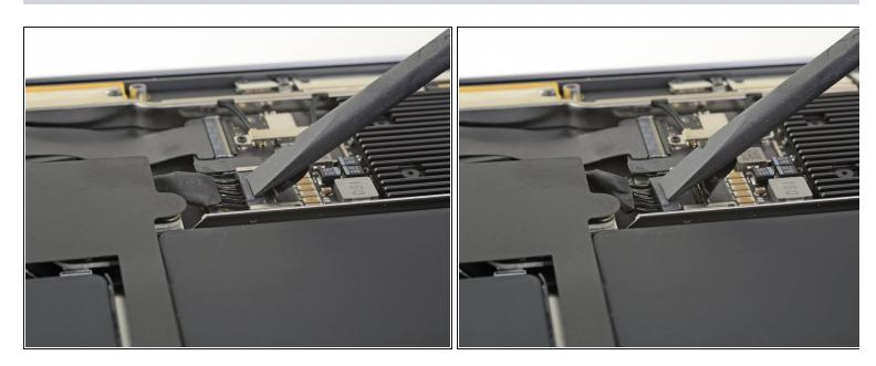
• Use a spudger to slide the battery connector parallel to the logic board and out of its socket on the logic board.
