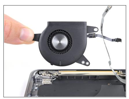
• Lift the fan out of the case to remove it.
