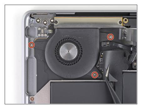
Use a T4 Torx driver to remove the three 2.7 mm screws securing the fan.
