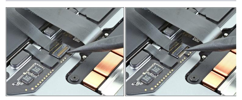
• Use the pointed end of a spudger to lift up the small locking flap on the trackpad cable's <u>ZIF</u> connector.
