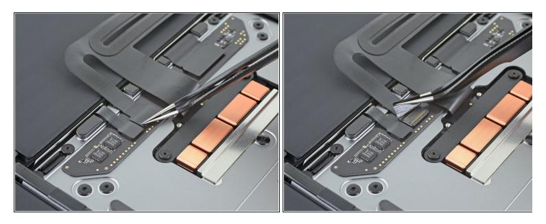
Use a pair of tweezers to peel back the tape covering the trackpad cable connector.
