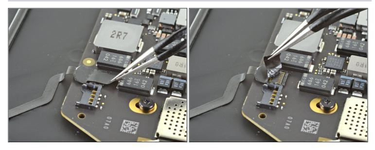
• Use a pair of tweezers to peel back the tape covering the microphone cable connector.
