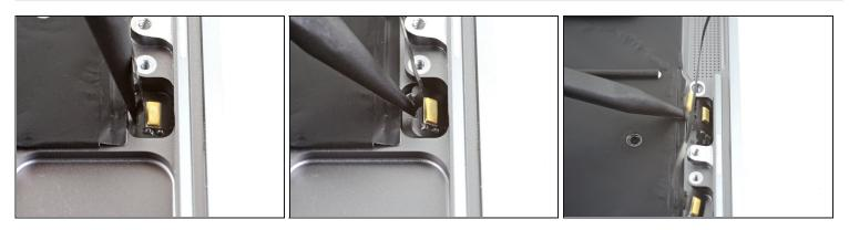
• Use the pointed end of a spudger to carefully pry one of the remaining microphones out of its recess in the upper case.
