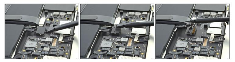
• Use the flat end of a spudger to pry up and unlatch the metal locking arm on the battery connector.
