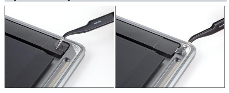
• Use a pair of tweezers to peel back the black pull tab on the speaker's stretch-release adhesive until you can grip it with your fingers.
