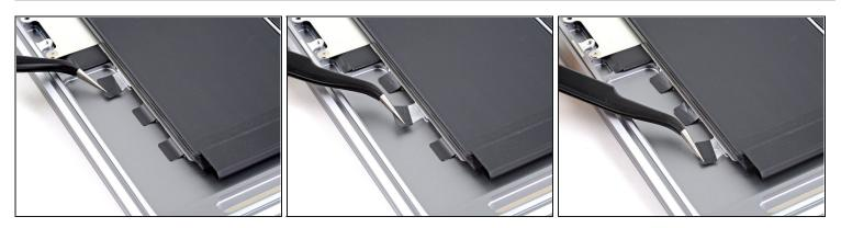
The MacBook's battery cells are attached to a metal tray as a complete assembly, which is adhered to the case with a total of six stretch-release adhesive strips.
