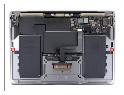
Use a T3 Torx driver to remove the two 2.6 mm screws securing the battery tray to the case.
