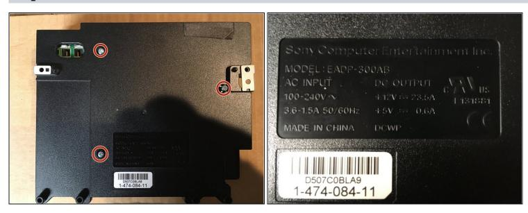
• Remove 3 Phillips screws from the bottom of the power supply. These hold together the upper and lower halves of the plastic power supply case.
