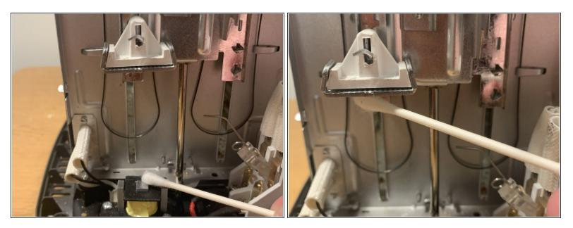
• After the shell is removed, take a cotton swab and clean the electromagnets that allow the lever to stay down.
