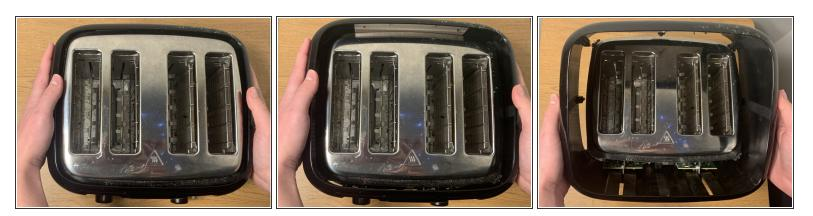
• Carefully remove the shell of the toaster by lifting up to get to the inside.
