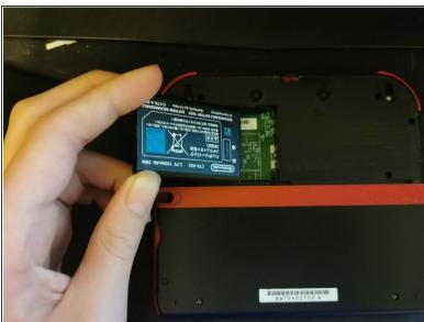
Lift up the battery and remove it.
