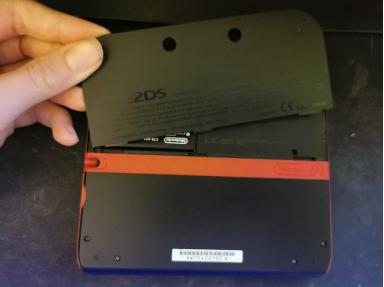
Lift the battery cover up and pull it out.
