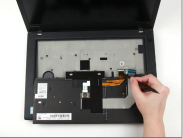
Use the flat end of a spudger to flip up the locking flaps securing each of the two ribbon cables.
