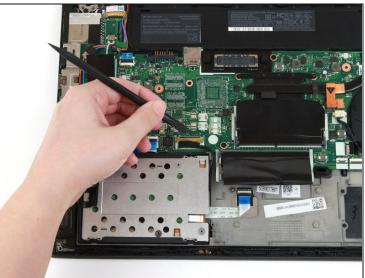
• Use the flat end of a spudger to flip up the metal clip securing the SSD connector to the motherboard.
