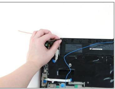
• Use your fingers to lift the LCD cable out of its slot.
