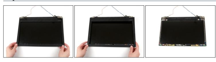
Use both hands to lift the bezel up and away from the display assembly.
