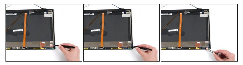
• Use a pair of blunt nose tweezers to peel the copper tape off of the hinge frame.
