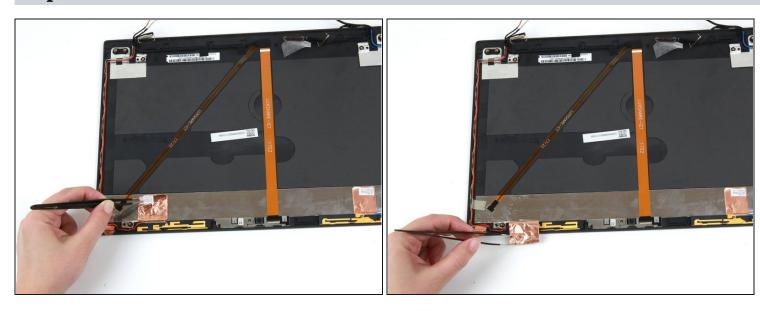
• Use a pair of blunt nose tweezers to peel the copper tape up from the display assembly in the bottom left-hand corner.
