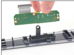
• Lift the USB board straight up to remove it from the interactive band.
