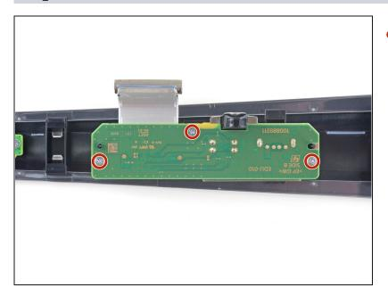
Use a Phillips screwdriver to remove the three 6.5 mm-long screws securing the USB board.
