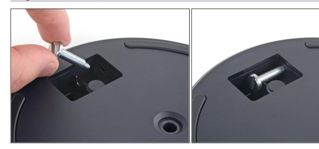
• Insert the screw into the cubby on the bottom of the stand.
