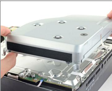
• Lift the optical drive away from the device to remove it.
