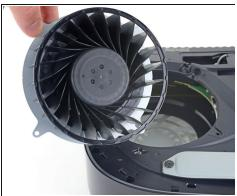
• Lift the fan up and out of the case to remove it.
