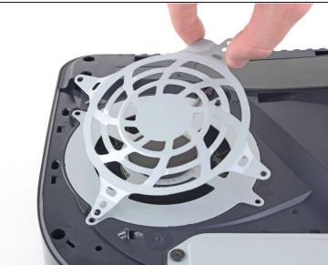
• Lift the fan shroud straight up to remove it.
