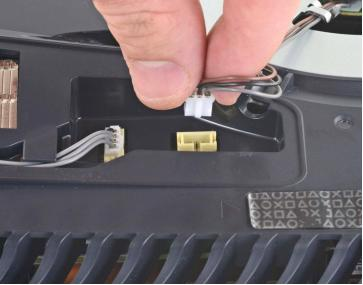
• Use your fingers to grip the edges of the fan cable connector, and pull up to disconnect it from the motherboard.
