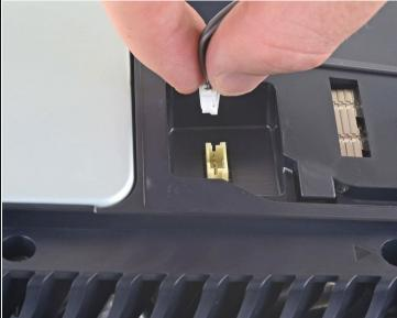
Use your fingers to grip the edges of the optical drive cable connector, and pull up to disconnect it from the optical drive.
