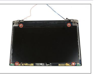
• Use a Phillips #1 screwdriver to remove the four 3 mm screws from each corner of the screen.
