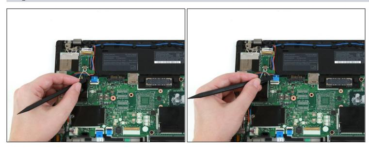
• Use the flat end of a spudger to slide the power button cable out of its connector on the motherboard.
