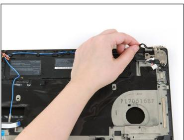
• Use your fingers to remove the camera cable from its slot.
