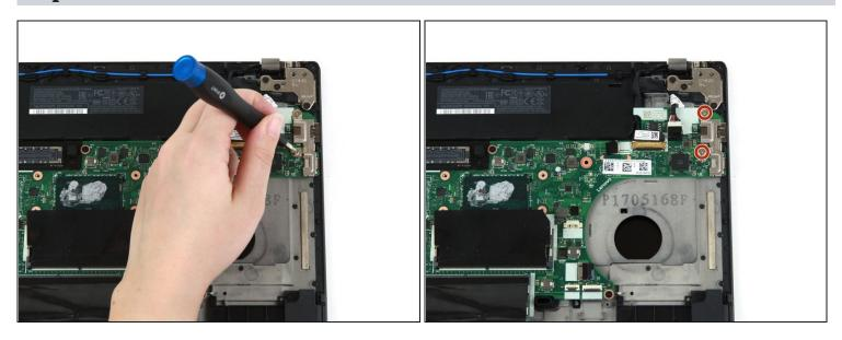
• Use a Phillips #1 screwdriver to remove the two 4 mm screws from the USB bracket.
