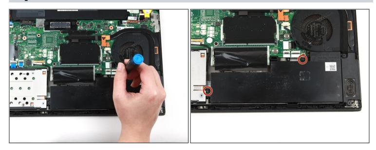
• Use a Phillips #1 screwdriver to remove two 5 mm screws from the internal battery.
