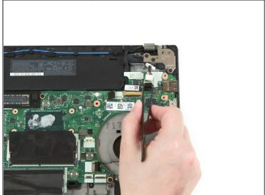
• Use a pair of blunt nose tweezers to disconnect the DC-in cable from its socket on the motherboard.
