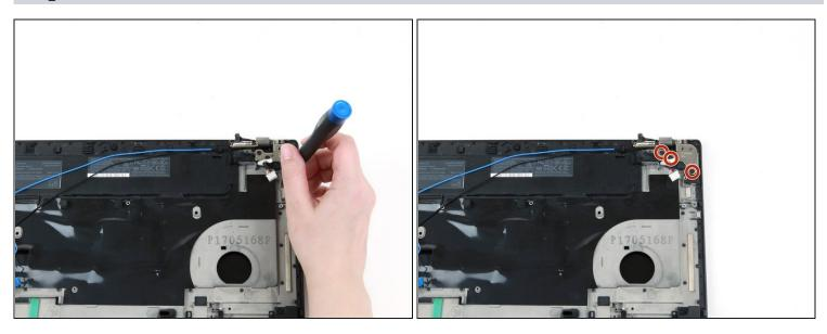
• Use a Phillips #1 screwdriver to remove three 4.5 mm screws from the hinge in the upper right corner.
