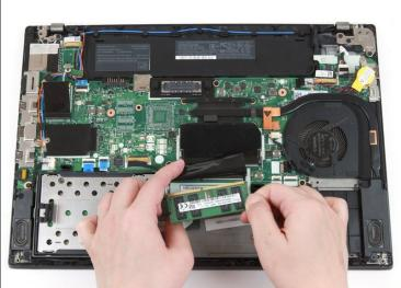
• Use your fingers to lift the RAM out of its socket and away from the laptop to remove it.
