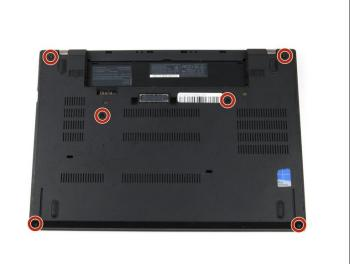
• Use a Phillips #1 screwdriver to loosen the six captive screws on the bottom cover of the laptop.
