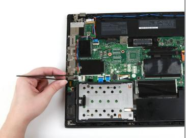
• Use a pair of blunt nose tweezers to remove the speaker connector from its socket.
