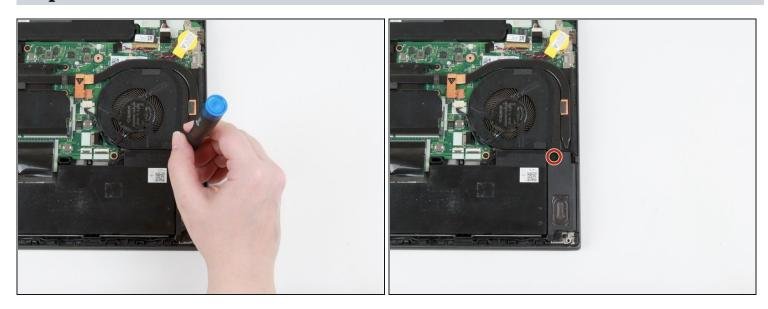
• Use a Phillips #1 screwdriver to remove the single 5 mm screw from the speaker to the right of the internal battery.
