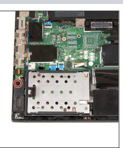
• Use a Phillips #1 screwdriver to remove the single 5 mm screw from the speaker to the left of the SSD.
