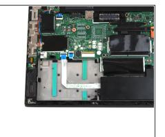
• Grab the tab on the left side of the SSD assembly, and pull up to remove it from the laptop.
