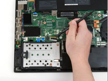
Use the flat end of a spudger to flip up the metal clip securing the SSD connector to the motherboard.
