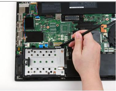
Use the flat end of a spudger to separate the connector from its socket.
